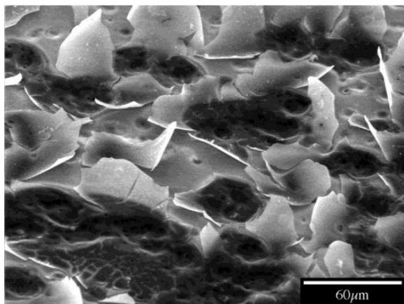
Figure 7. Biocorroded Ge surface; not yet crystallized
