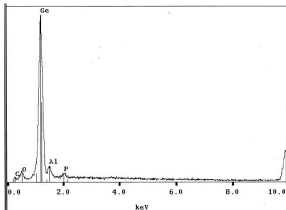
Figure 8. EDX-ray elemental analysis of initial deposit (note trace carbon and phosphorous components)
