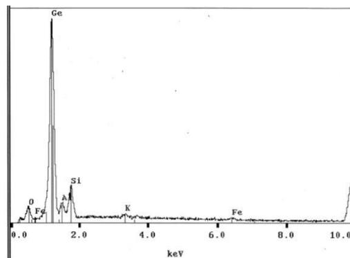
**Figure 4.** EDX-ray elemental analysis of Taicho stone on Ge in Figure 2
