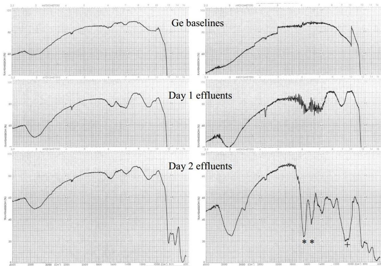
**Figure 6.** IR spectra of effluents from devices without (left) and with (right) Taicho stone. Controlled volumes of the effluents were evaporated on Ge test plates prior to analysis. Note glycoproteinaceous character of Taicho stone slime effluent (\* Amide I & II, + carbohydrate).
