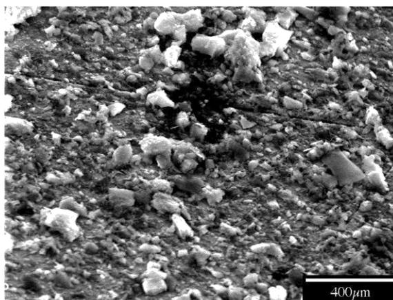
**Figure 2.** Taicho stone from water filter, spread over germanium surface
