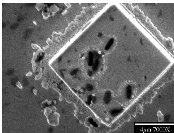
**Figure 1.** Scanning electron micrograph of live bacteria in GeO<sub>2</sub> microcrystal
