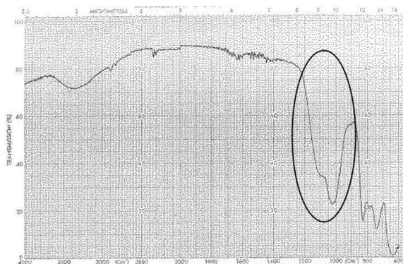
**Figure 3.** Internal reflection IR Spectrum of Taicho stone on Ge in Figure 2 (IR absorptions from stone are circled)
