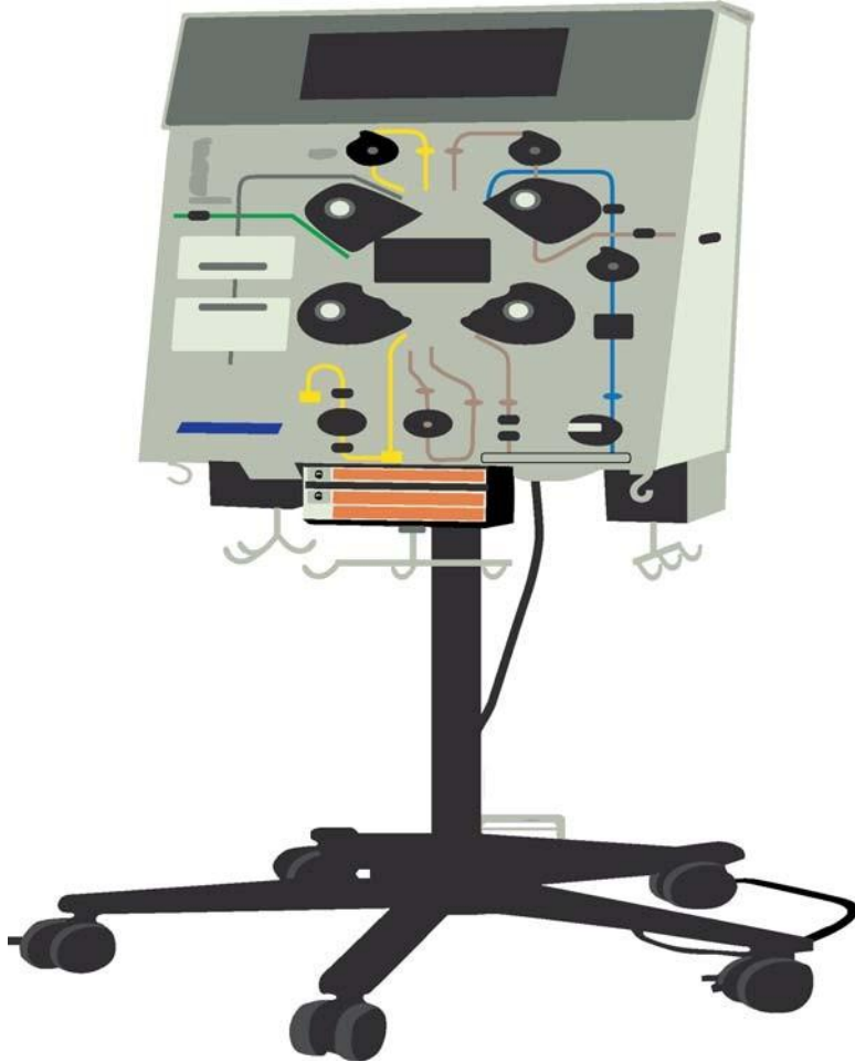
Figure 7 –CRRT machine in which all pumps are located on one platform and all dilution solutions and collection bags are also in one location hanging from poles and hooks. As above there are several manufacturers of such equipment.
