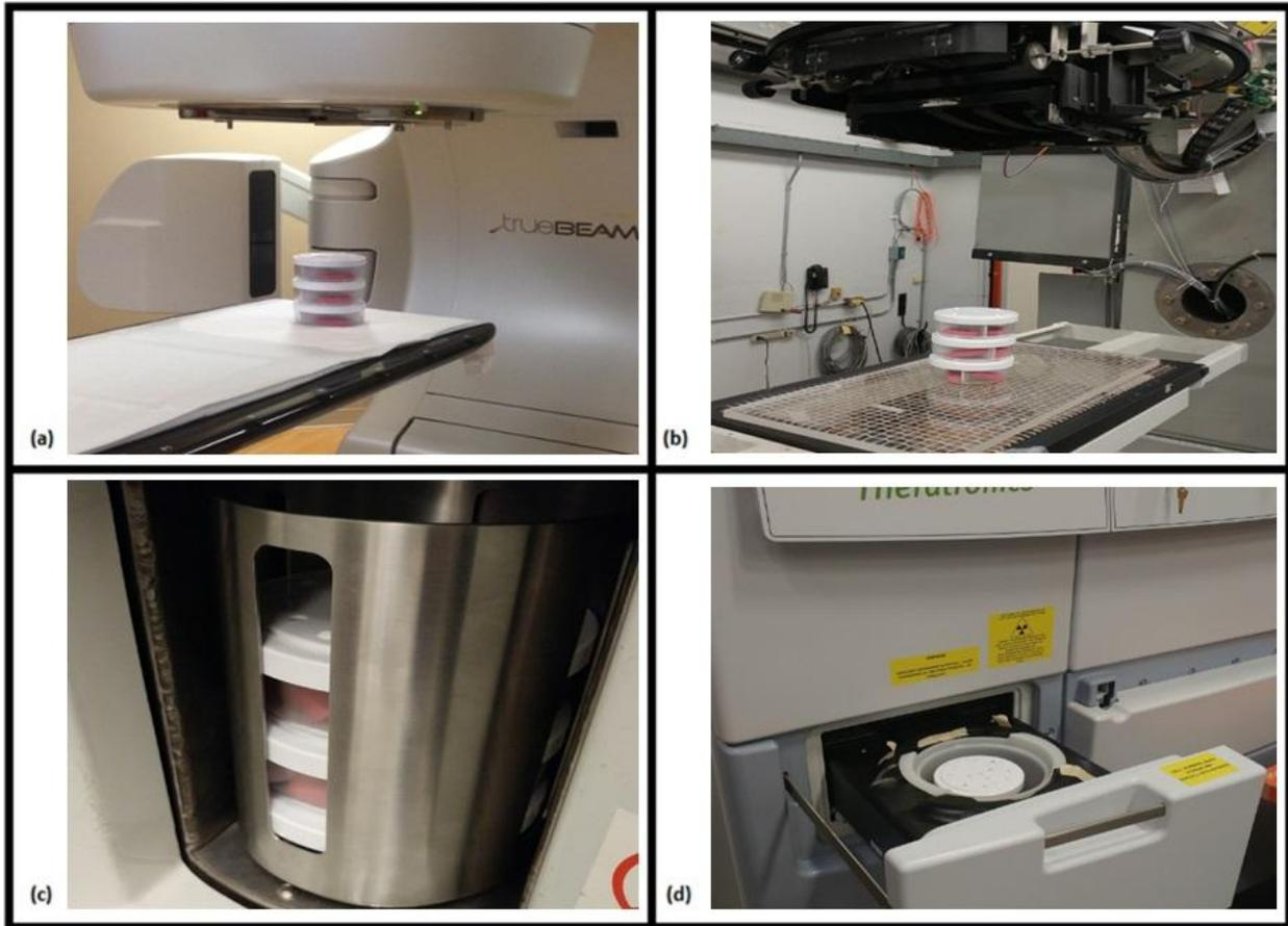
**Figure 2.** Set-up geometry for all testing with pie cages; (a) Varian Medical Systems, Inc.® TrueBeam® particle accelerator, (b) Best® Theratronics, Ltd.™ Equinox 100 Cobalt-60 unit, (c) Best® Theratronics, Ltd. GammaCell® 1000 Elite Cesium irradiator, and (d) Best® Theratronics, Ltd. Raycell® MK2 KV irradiator
