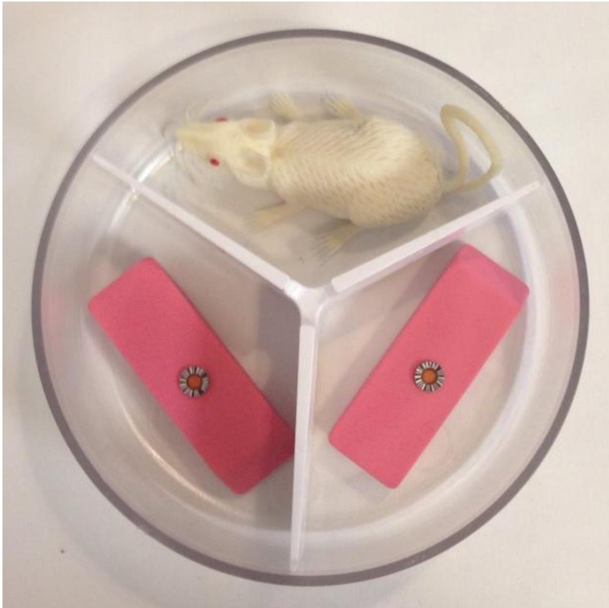
**Figure 1.** Localization of the TLD wafers on the mouse phantom.
