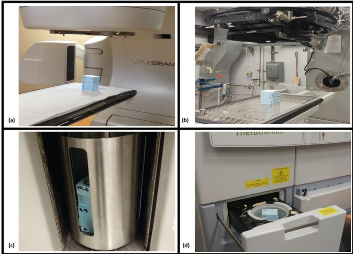
**Figure 3.** Set-up geometry for all testing without pie cages; (a) Varian Medical Systems, Inc.® TrueBeam® particle accelerator, (b) Best® Theratronics, Ltd.™ Equinox 100 Cobalt-60 unit, (c) Best® Theratronics, Ltd. GammaCell® 1000 Elite Cesium irradiator, and (d) Best® Theratronics, Ltd. Raycell® MK2 KV irradiator
