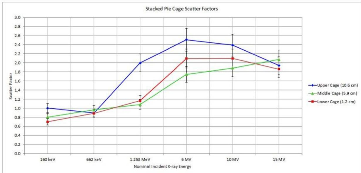
**Figure 4.** The average result projects the measurement for pie cage dosimetric net scatter at each level and energy. Dose to inserted mice can then be interpolated from these factors.
