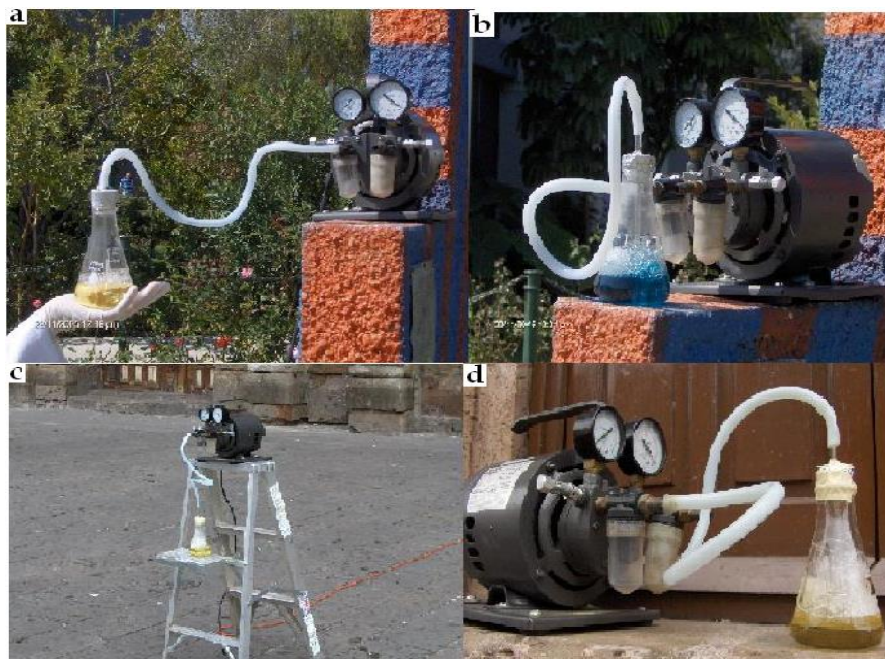
Figure 1. Method of bubbling dust from the air of Morelia with the vacuum pump (1,18,19) . (a) Bubbling in nutrient broth with sodium azide for the recovery of S. aureus , S. pyogenes , E. coli from the dust suspended and precipitate of the air outdoors of the UMSNH Garden. (b) Nutrient broth with methylene blue for enteric bacteria in dust suspended of air outdoor of the UMSNH Garden. (c) Nutrient broth with sodium azide dust from dust of the air outdoor in Valladolid Square and City Hall (d).
