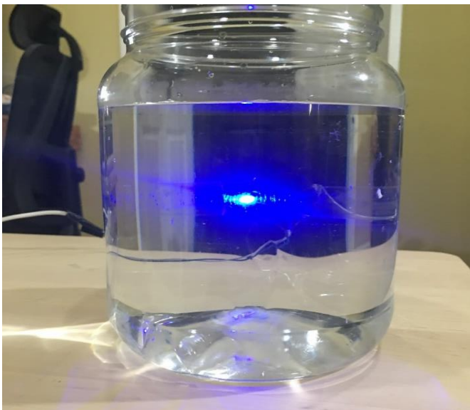
Figure 3: Clear mosquito bait with one blue LED
