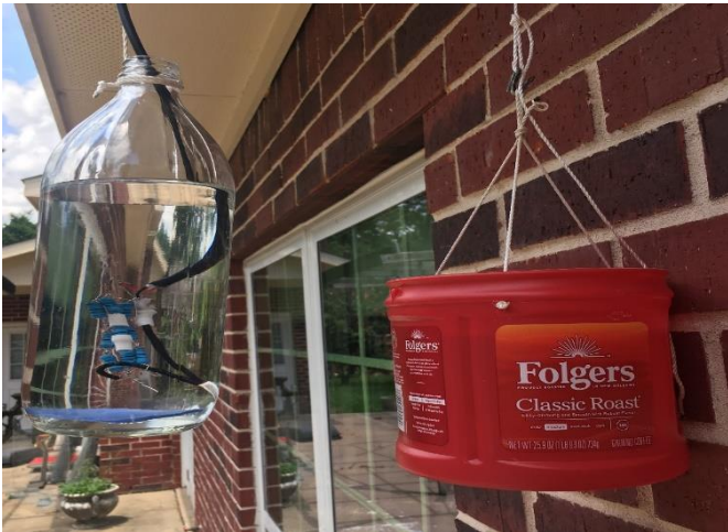
Figure 2: USB-powered female mosquito trap
