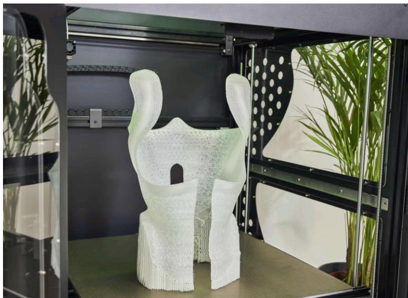
Figure 2.2 Kyphosis brace with variable density zones. courtesy of Create it REAL
