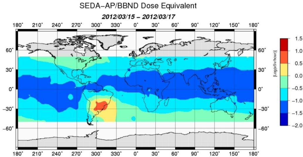
Figure 13. World map of neutron ambient dose equivalent rate distribution measured at SEDA (extra-vehicle) of ISS from March 15 to March 17, 2012 during no flare event on the courtesy of JAXA <sup>11)</sup>
