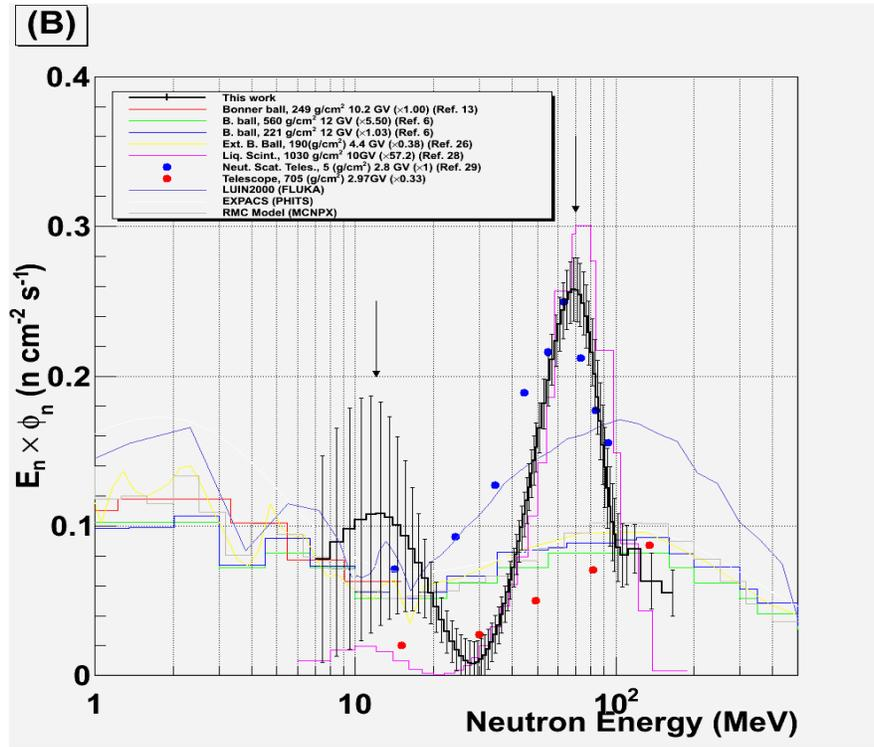
**Figure 10.** Measured neutron energy spectrum<sup>18)</sup> from 7 to 180 MeV at an altitude of 10.8 km compared with other calculated<sup>19,20,22)</sup> and measured<sup>23-27)</sup> spectra
