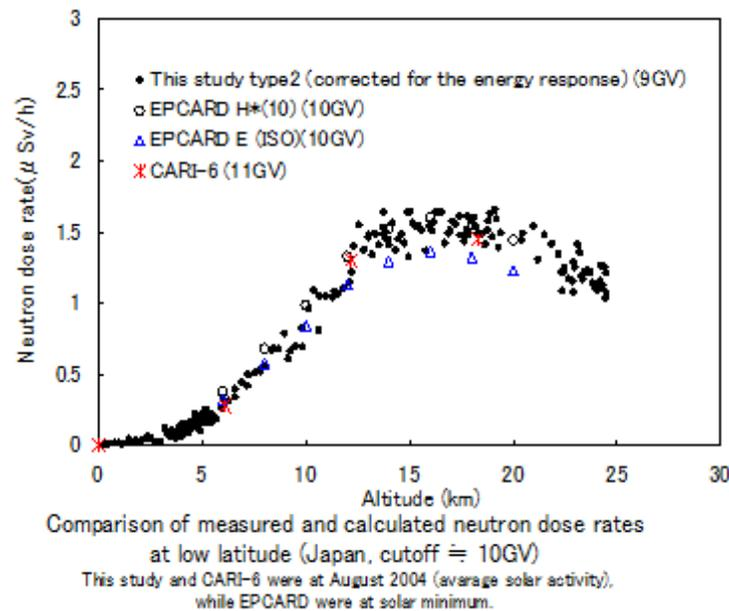
**Figure 17.** Altitude variation of measured neutron ambient dose equivalent rate <sup>11)</sup>, compared with calculated results <sup>28,29)</sup>
