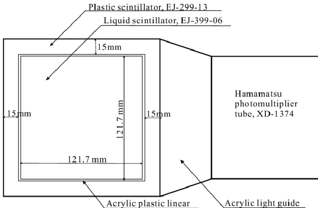
**Figure 1.** Configuration of phoswich detector<sup>1-3)</sup>
