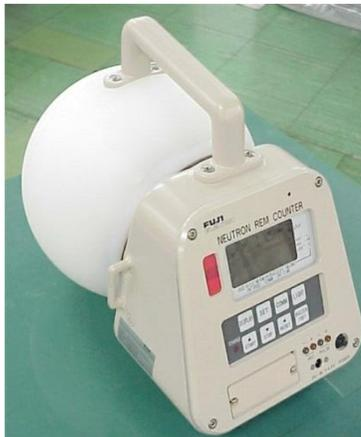
**Figure 6 (b).** Outlook of high-efficiency neutron dosimeter, NSN2 <sup>5,6)</sup>
