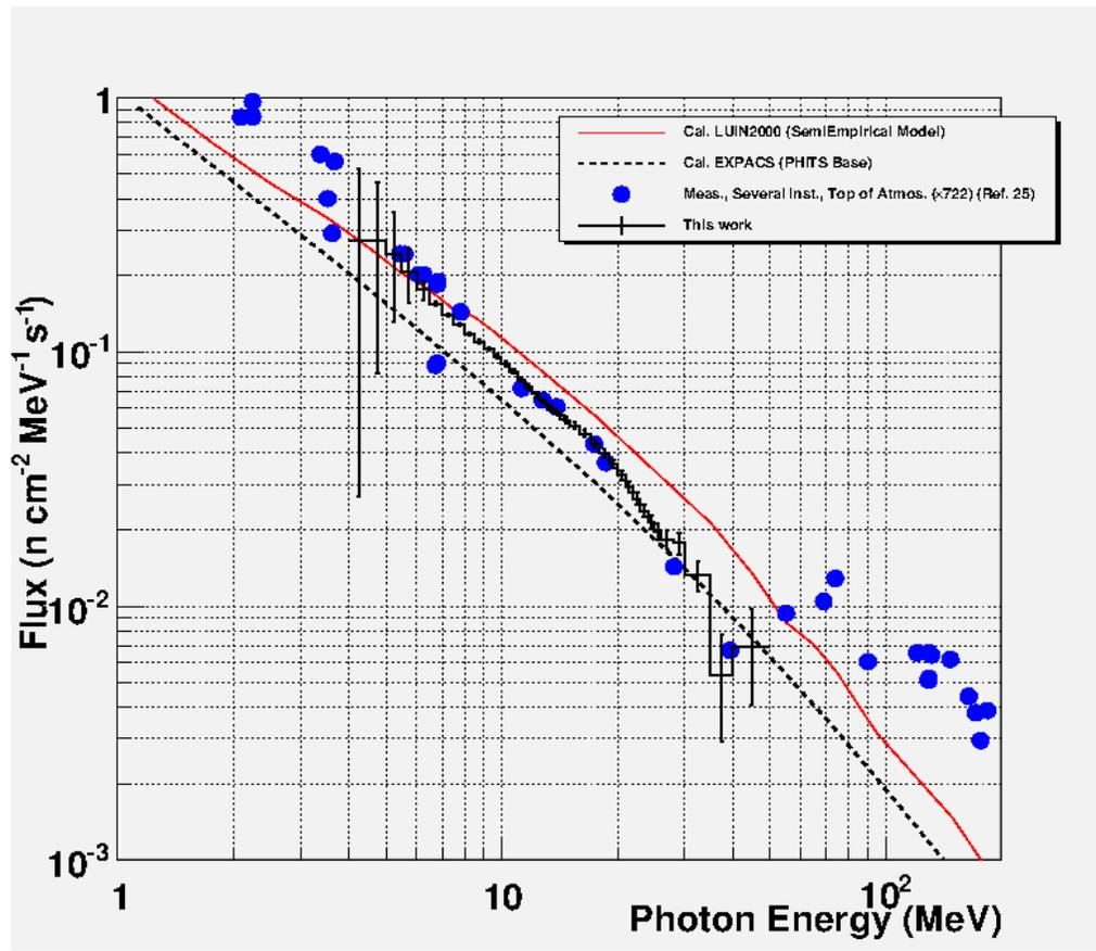
**Figure 9.** Measured photon energy spectrum<sup>18)</sup> from 4 to 50 MeV at an altitude of 10.8 km compared with other calculated<sup>19,20)</sup> and measured<sup>21)</sup> spectra
