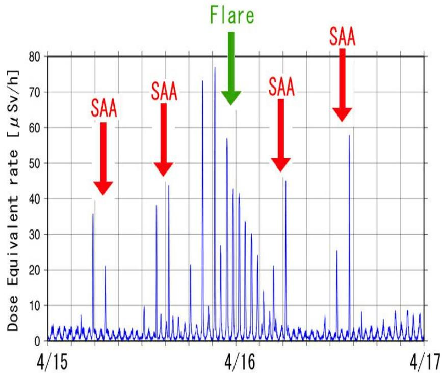
**Figure 15 (b).** Time variation of neutron ambient dose equivalent rate in the US module at ISS when a big solar flare on April 16, 2001 was observed in the polar region <sup>8,9)</sup>
