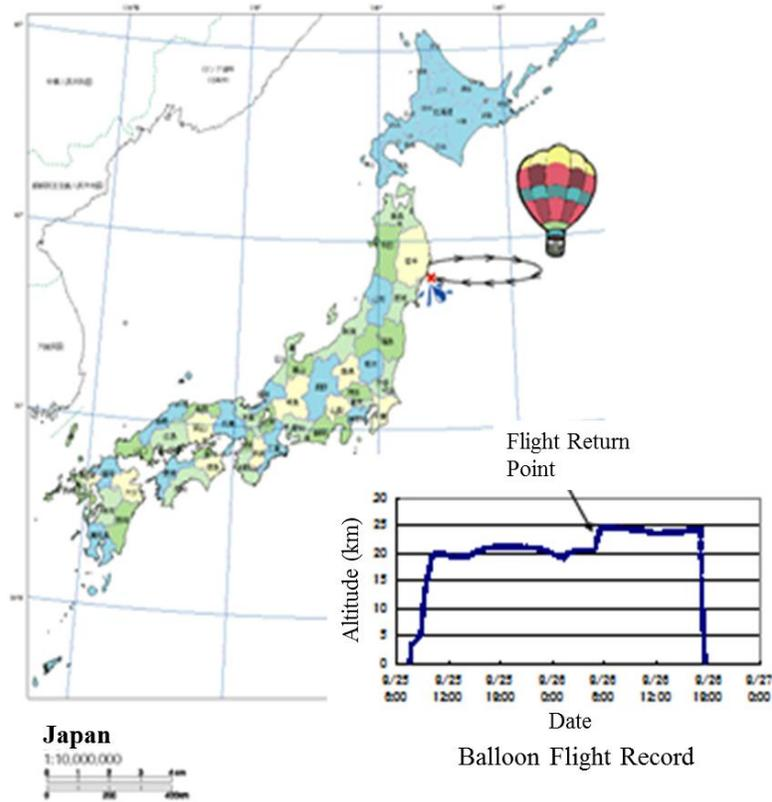
**Figure 16.** Flight route of the balloon experiment at Sanriku, Japan on August 25, 2004. <sup>12)</sup>
