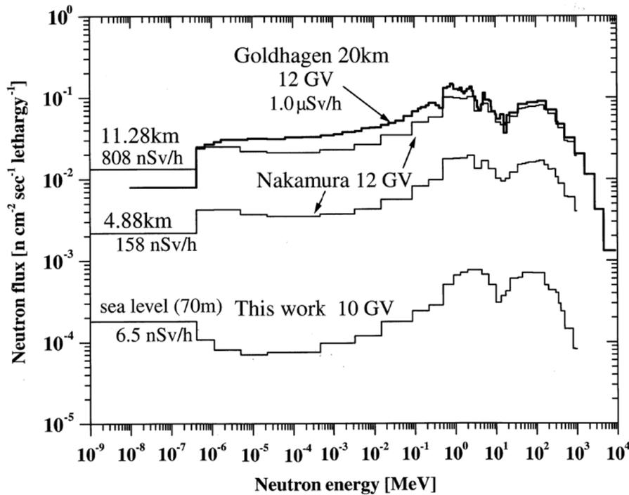
**Figure 11.** Cosmic-ray neutron energy spectra in lethargy unit at different atmospheric depths (altitudes) around the high cutoff rigidity of 10 to 12 GV obtained by Goldhagen et al.<sup>23)</sup> in June 1997 (solar minimum period) and Nakamura et al.<sup>25)</sup> on February 27, 1985 (solar minimum period), both on board the airplane, together with the average value at sea level in Sendai, Japan (10 GV) on September 2, 2002 (solar maximum period) by Nakamura et al.<sup>26)</sup>
