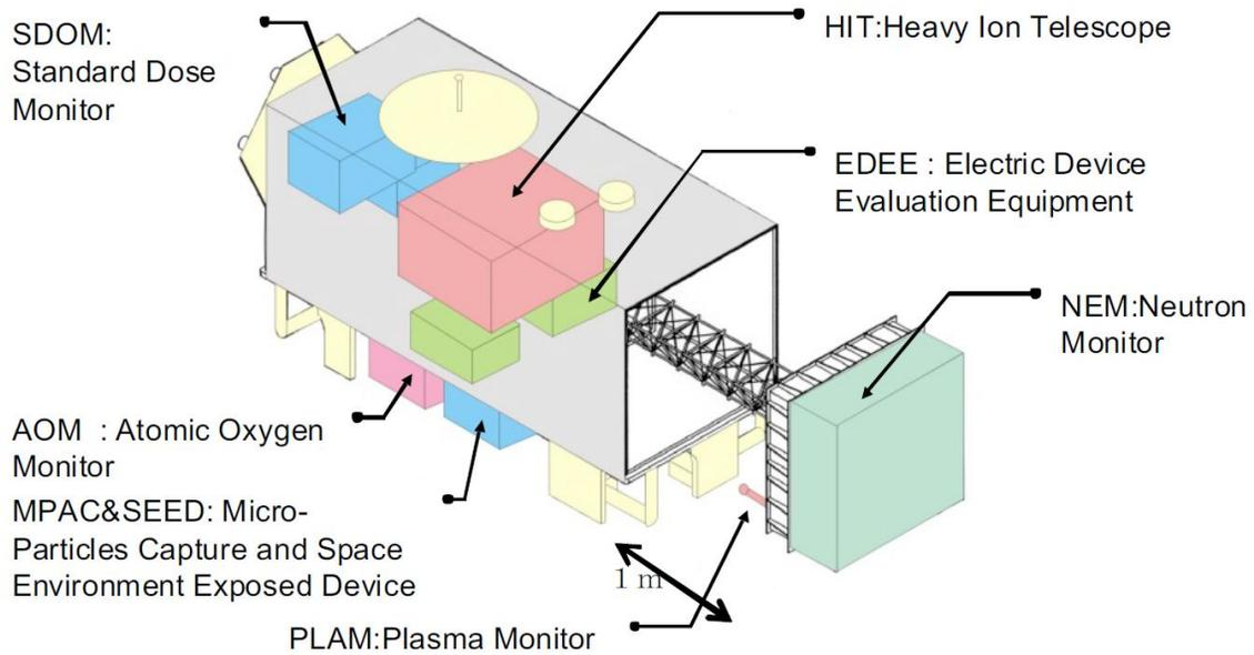
**Figure 5.** The gross feature of SEDA (Space Environmental Data Acquisition equipment – Attached Payload) <sup>10,11)</sup>
