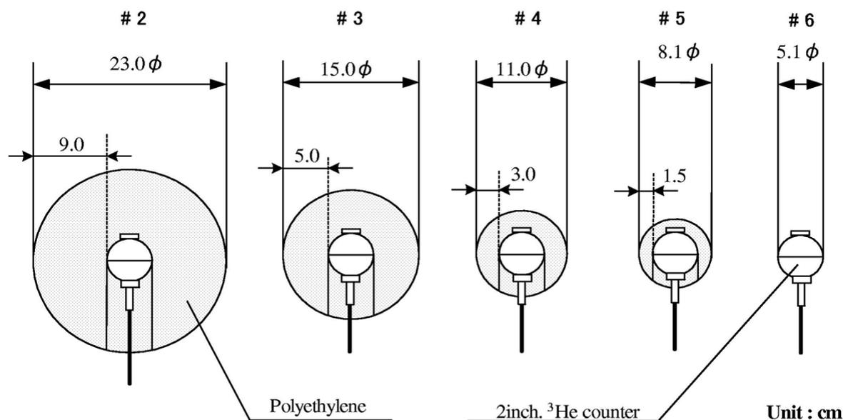
**Figure 2.** Cross sectional view of Bonner sphere detector <sup>4)</sup>
