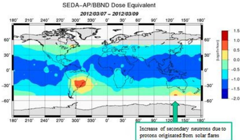
Figure 14. World map of neutron ambient dose equivalent rate distribution measured at SEDA (extra-vehicle) of ISS from March 7 to March 9, 2012 during flare event on the courtesy of JAXA <sup>10,11)</sup>
