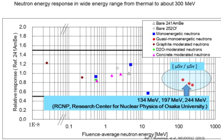
**Figure 18.** Neutron ambient dose equivalent response relative to the response to <sup>241</sup>Am-Be neutron source of lightweight dosimeter, NSN3, over wide energy range from thermal to 300 MeV <sup>7)</sup>
