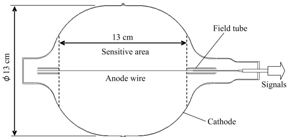
**Figure 7 (a).** Cross-sectional view of lightweight neutron dosimeter, NSN3<sup>7)</sup>
