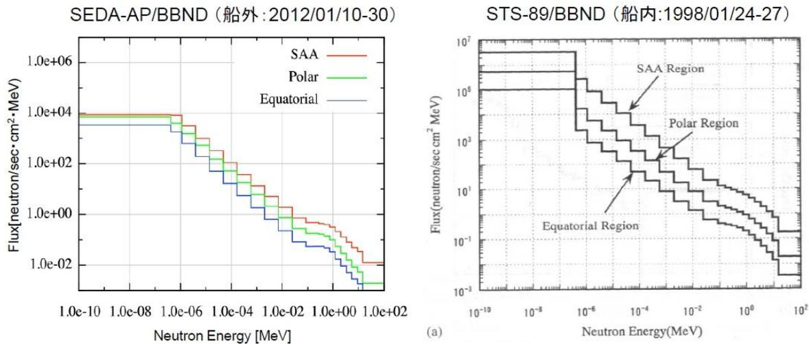
**Figure 12.** Comparison of neutron spectra obtained with BBND at SEDA (extra vehicle) in January 10 to 30, 2012 on the courtesy of JAXA and at STS89 in space shuttle vehicle in January 24 to 27, 1998<sup>8,9)</sup>.
