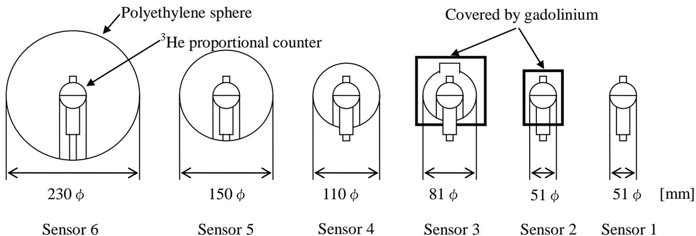
**Figure 3.** Cross sectional view of BBND sensors<sup>8)</sup>
